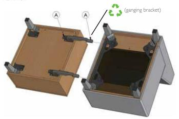
A: Separate the table from the chair by squeezing the quick release button at one end of the ganging bracket and slide the two apart by about an inch. Repeat this procedure with the second ganging bracket; the chair and table can now be pulled fully apart. Remove the ganging bracket from the neighbor.
