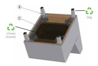
**B & C:** Now turn the seat upside down. Using the Philips screwdriver, remove the legs and chassis brackets from the seat box.
