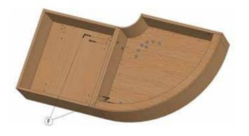
**F:** Using the Philips screwdriver, remove the four screws holding the tables together.
