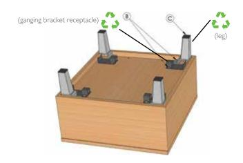
**B & C:** Now flip the table over and using the Philips screwdriver, remove the legs and ganging bracket receptacles. Next using the flat blade screwdriver and hammer, remove the plastic glides from the bottom of each leg.
