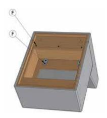
F: Using the Philips screwdriver, remove the screws securing the back retainer brackets and the three screws attaching the seat box to the back box.
