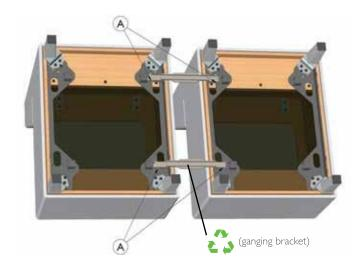
A: If two or more chairs are ganged together, they should be separated from their neighbor first. To do this squeeze and hold the quick release button at one end of the ganging bracket and push the two seats apart by about an inch. Repeat this procedure with the second ganging bracket; the seats can now be pulled fully apart. Remove the ganging bracket from the neighbor:
