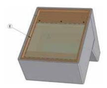
**E:** Take the knife or box cutter and carefully slice the dust cover alongside the staples attaching it to the seat box.
