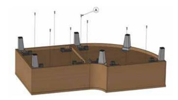
**A:** Using the Philips screwdriver, remove the four screws as shown above.
