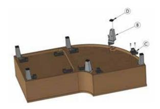
**B - D:** Using the Philips screwdriver, remove the legs and ganging bracket receptacles (with ganging brackets if present). Next using the flat blade screwdriver and hammer, remove the plastic glides from the bottom of each leg.
